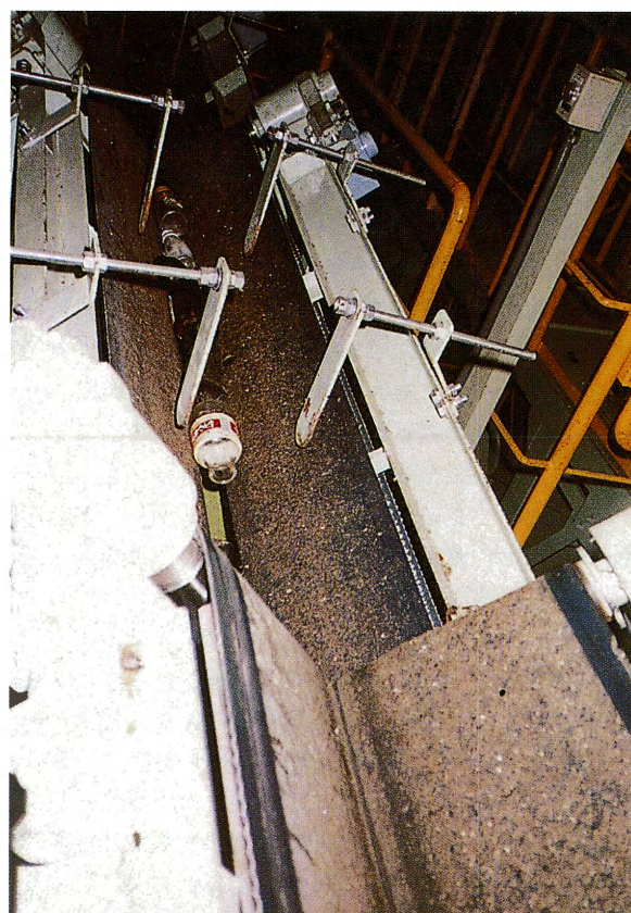
図8 引離しコンベヤ上を流れるガラス瓶 Fig.8 Glass bottles on V-belt conveyor
