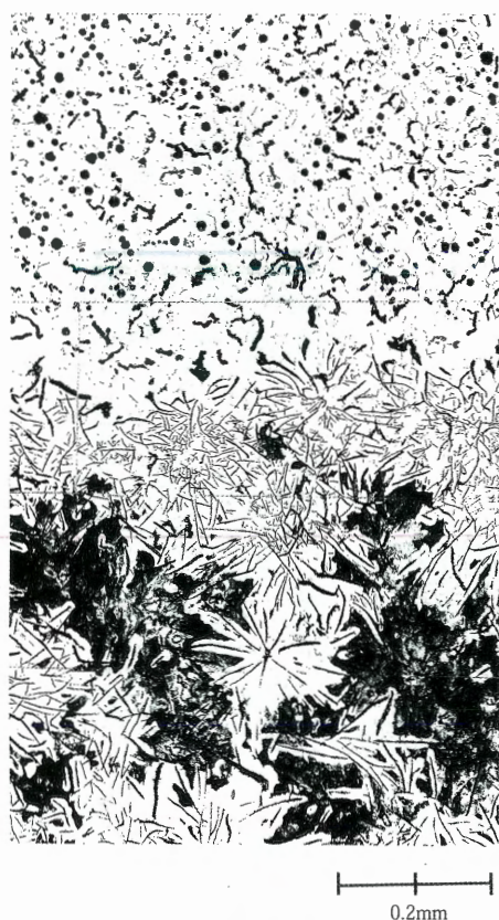
図5 黒鉛遷移組織 Fig. 5 Alteration structure of graphite morphology
