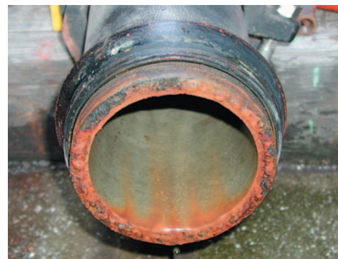
図12 非防食部(3年経過後) Fig. 12 Non-corrosion prevention part of cutting section (Passes in three years)
