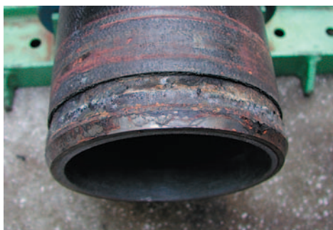
図11 防食部(3年経過後) Fig. 11 Corrosion prevention part of cutting section (Passes in three years)
