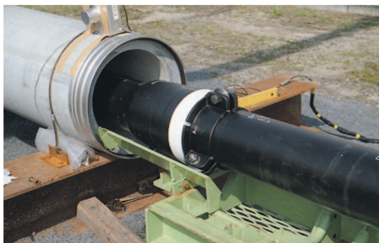
図14 直線管路での施工試験 (NS形) Fig. 14 Construction test into straight line casing pipeline (NS-type joint)
