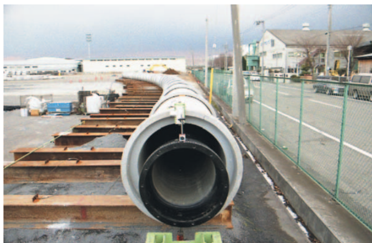
図13 S字カーブ管路での施工試験 (S形) Fig. 13 Construction test into S-curve casing pipeline (S-type joint)
