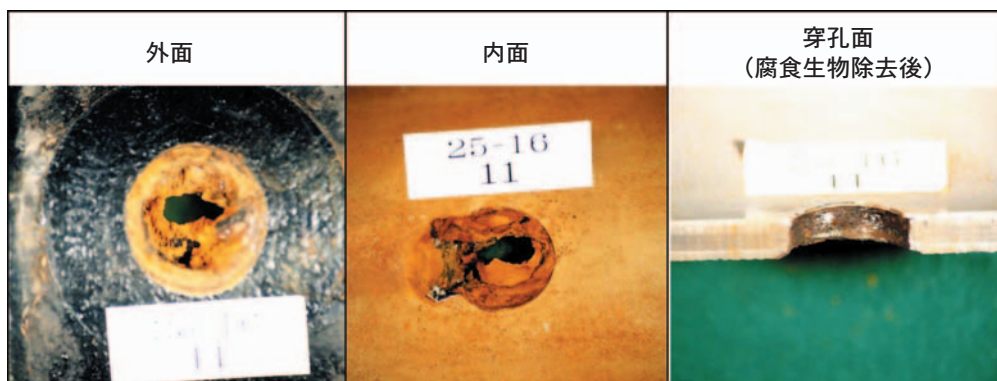
図21 穿孔部の腐食状況(防食なし) Fig. 21 Corrosion situation of drilling part (No corrosive protection)
