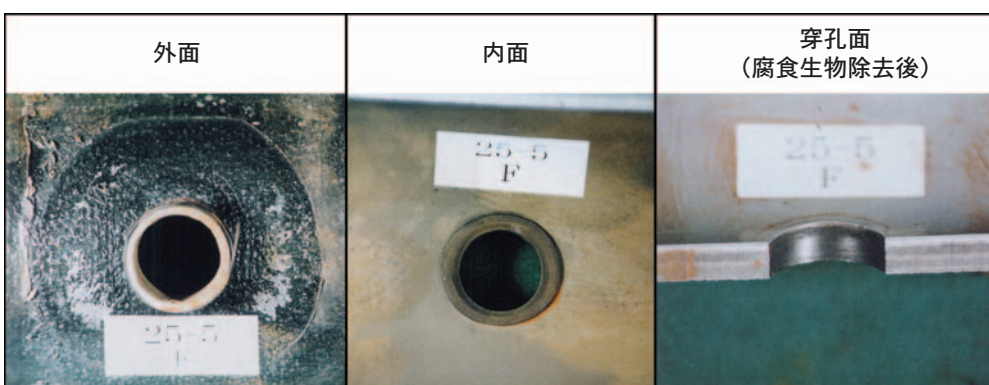
図24 穿孔部の腐食状況(ストレッチャ) Fig. 24 Corrosion situation of drilling part (Stretcher)
